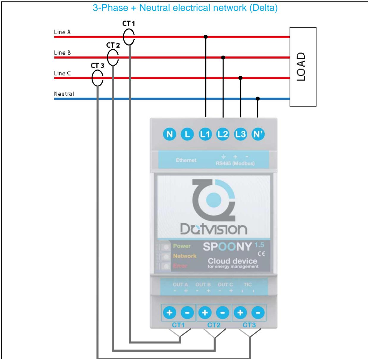
Notes: Schematics present current transformers but same schematic apply when using Rogowski Coils.
